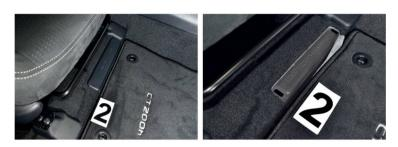
Fig. 7. The VIN of a Lexus CT 200h vehicle standardly placed below the front passenger's seat.
