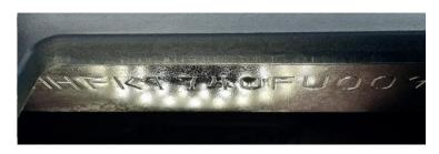
Fig. 4. Overall, the identifier is visually inaccessible even following this dismantlement. Reading the VIN is very uncomfortable, and the inclined surface plays a role as well
