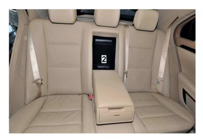
Fig. 6. A VIN located in a non-standard way in a Mercedes – Benz "S" class vehicle in the space behind the elbow rest of the rear seats. It occurs to hardly anyone to look for the identifier there. On the other hand, this space is clean, dust-free so the identifier is not exposed to the negative effects of ambient phenomena
