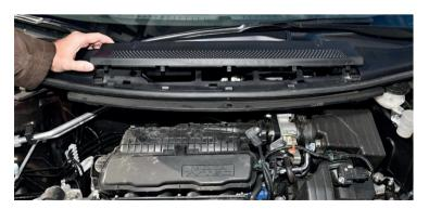
Fig. 3. Demonstration of a dismantled plastic cover in the space in front of the windscreen wipers
